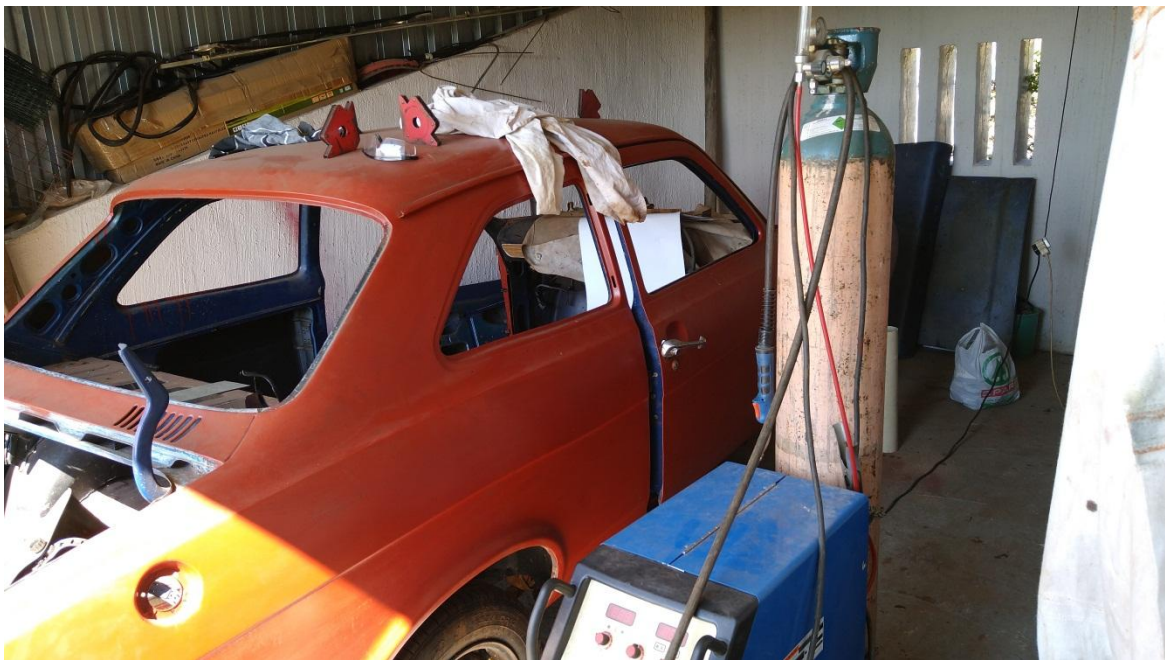
A bit of welding required mainly in the boot and floor
