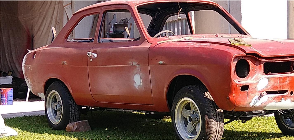
Some more body filler in the dents I could not get out.
