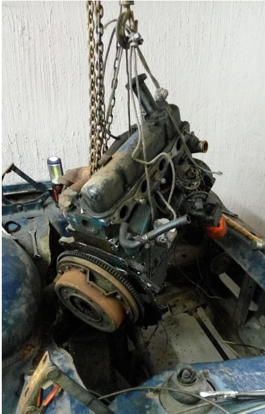
The original engine was a 1300. I am not into originality so I am putting in a 1600 GT engine with twin weber carb.
