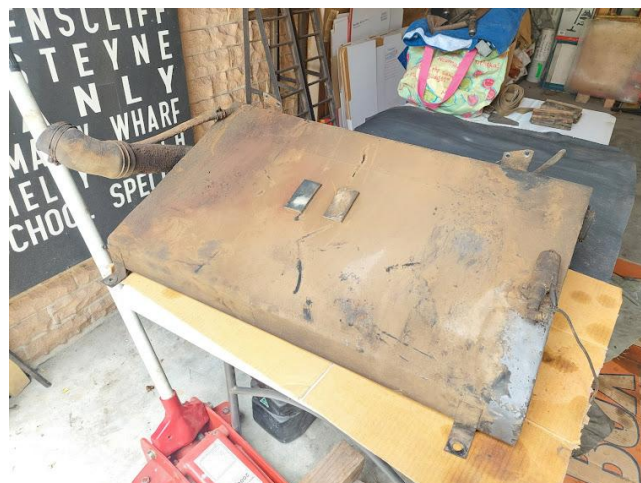
Very dusty petrol tank showing signs of leaks from the filler hose and the petrol reserve tank solenoid.
