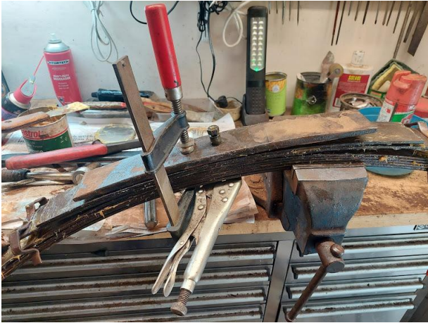
Reassembling a spring using two leaves from the spare
