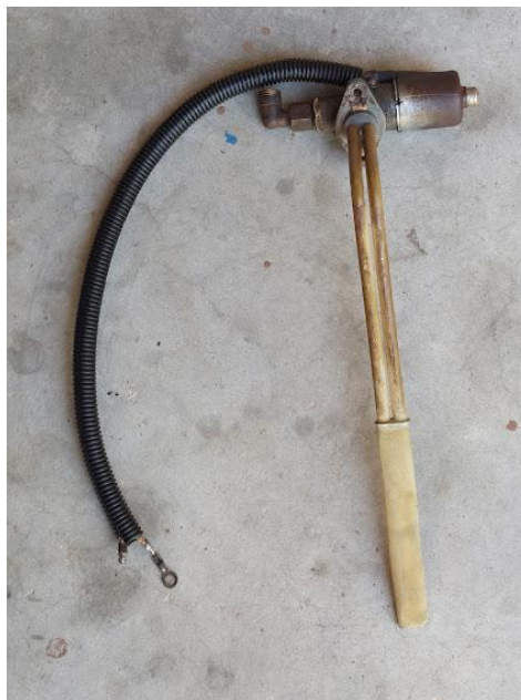
Refurbished, rewired and tested petrol reserve solenoid.
